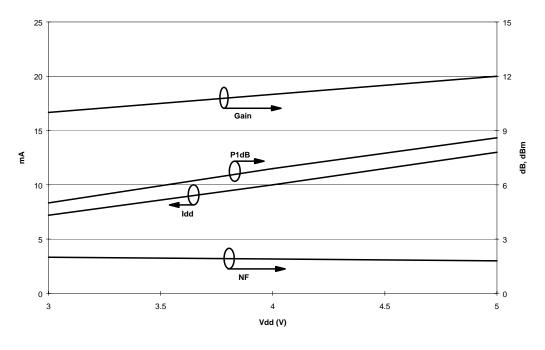
Typical Characteristics -  $V_{DD}$  = 5.0 V
